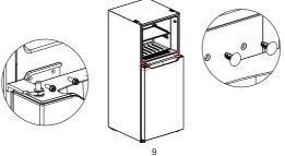
7) Take out the left upper hinge, left upper hinge cover, and right decorative cover from the accessory bag, install the freezer door on the middle hinge, and install the left upper hinge, left hinge cover and hole cap. Finally, install the right decorative cover on right side of end cap of freezer door..
