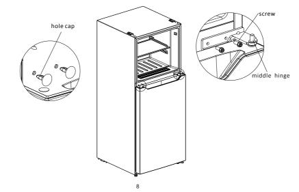
4)Remove the lower hinge assembly from lower right corner and remove the hole cap, screw cap from lower left corner; Dismantle the hinge shaft and adjustable foot and install them on other side of lower hinge; then install the lower hinge assembly on lower left corner by fitting screws, and install the hole cap and screw cap on lower right corner.
