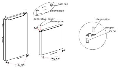
6) Install the Refrigerator compartment door on the lower hinge and then install the middle hinge andhole caps.
