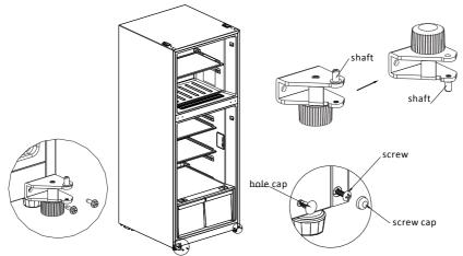
5)Dismantle the stoppers, sleeve pipes of both refrigerator door and freezer door, install them on the other side of both doors; exchange the installation position of sleeve pipe and hole cap on upper end cap of refrigerator door; remove the left decorative cover of freezer door, and move the sleeve pipe
